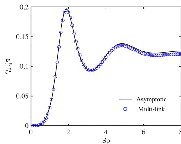
Fig. 6 The propulsive thrust  $F_p/\varepsilon^2$  generated by an elastic filament oscillated harmonically at one end as a function of the sperm number  $Sp$  with  $\varepsilon = 0.1$ . Numerical results from the multi-link model with  $N = 50$  (blue circles) display satisfactory agreements with previous asymptotic results based on a continuum description of the elastic filament<sup>36</sup> (black solid line).
