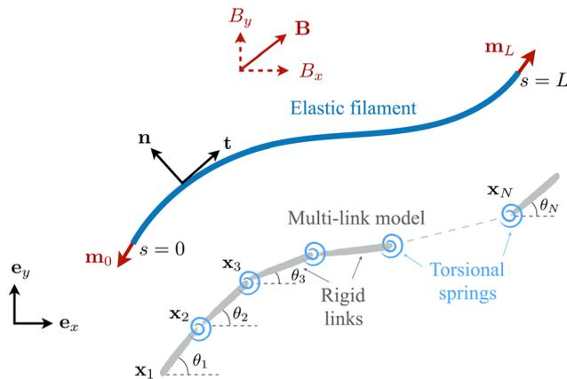
Fig. 2 Schematic diagram of an elastic filament with prescribed magnetic moments ( $\mathbf{m}_0$  and  $\mathbf{m}_L$ ) at its two ends under an oscillating external magnetic field  $\mathbf{B}$ . The elastic filament is discretized by a chain of rigid links connected by torsional springs.
