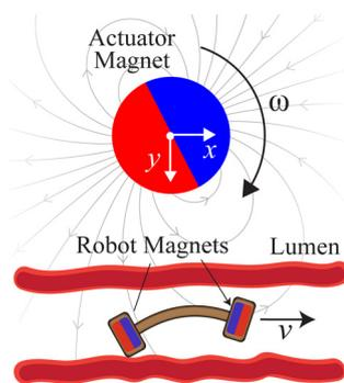
**Fig. 1** A soft endoluminal robot comprises a compliant continuum structure with two embedded magnets of opposite polarity. Its locomotion is actuated by an external magnetic field. The soft robot can travel through lumens of the body for potential biomedical applications. Reproduced with permission<sup>26</sup>. Copyright 2020, IEEE.
