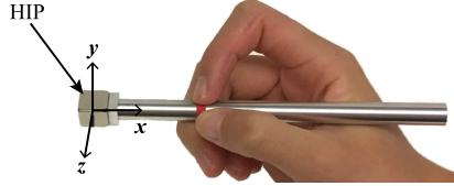
Fig. 1. Stylus of the untethered magnetic haptic interface used in the original study [1], held in a precision pen-hold grasp. Forces and torques are applied at the haptic interaction point (HIP). The coordinate system used defines  $x$  along the stylus,  $y$  pointing upward, and  $z$  pointing toward the subject when the stylus is held in front of the subject as shown. This coordinate system should be viewed as constant in the frame of the hand, not the stylus.
