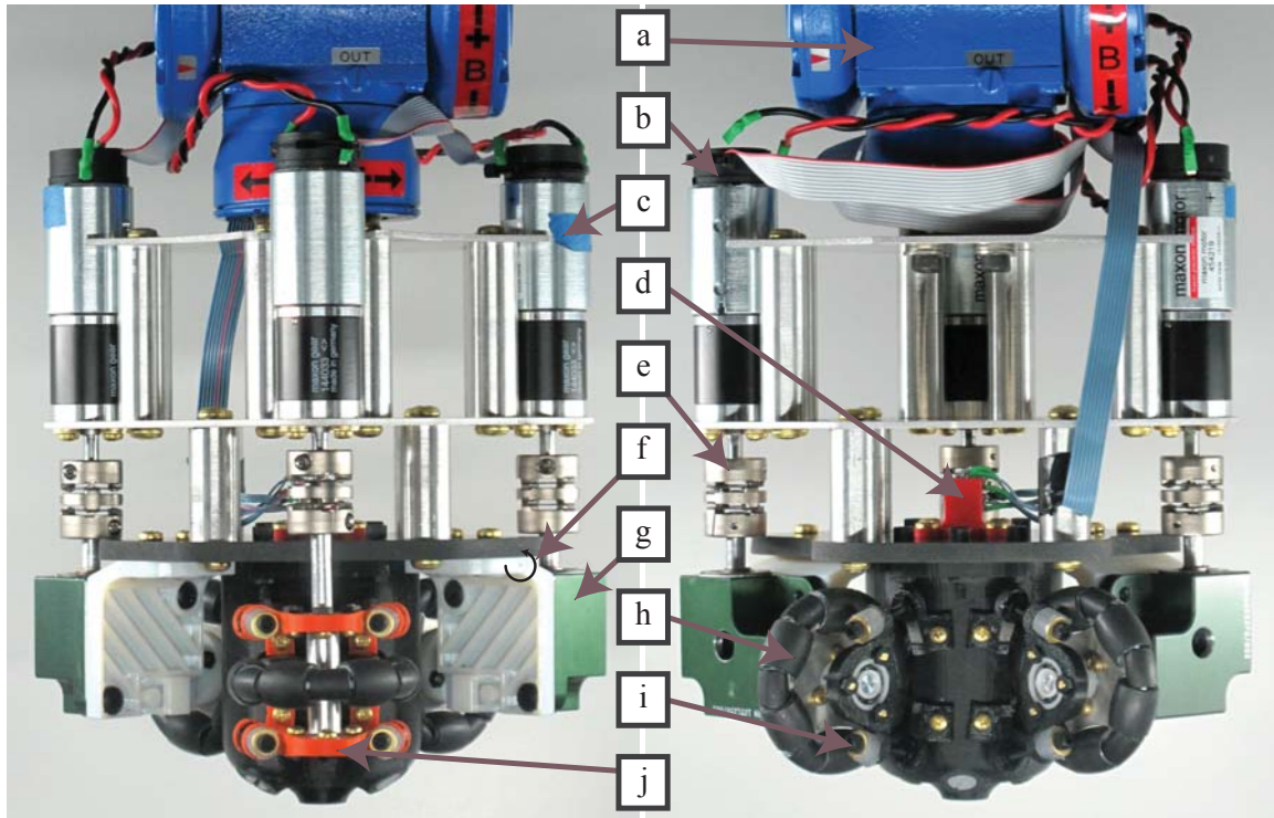
Figure 3.7. Prototype SAMM shown mounted to the tool frame (a) of robotic manipulator. Encoders (b) measure the gearmotors' (c) position. The cluster of Hall-effect sensors (d) measures the spherical magnet's dipole. Power is transmitted through aluminum helical shaft couplings (e) to omniwheel axles or 90° gearboxes (g), which pivot for omniwheel compliance (f). Omniwheels (h) are tensioned to the spherical magnet through adjustable spring-tensioned pillow blocks (i), whose tension can be manually tuned through adjustment screws (j).
