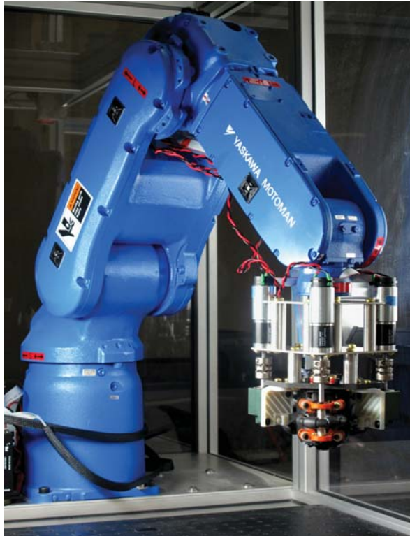
Figure 6.1. Experimental setup showing orientation and mounting of SAMM onto a 6-DOF Yaskawa Motoman robotic arm.
