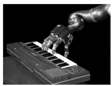
Figure 1. The DLR Hand II and Light-Weight Arm III playing the piano.
