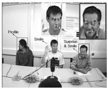
Figure 2. An example of head detection, feature extraction, and expression recognition.
