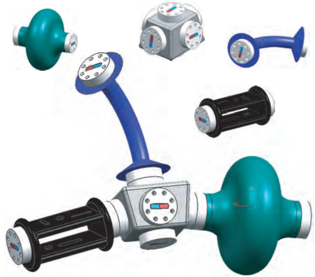
Fig. 1. Concept drawing of a modular microrobot. Relatively simple modules can be combined to form complex systems. The connection mechanism must allow for attraction and alignment of the modules to reduce control requirements and thus ensure robust self-assembly.
